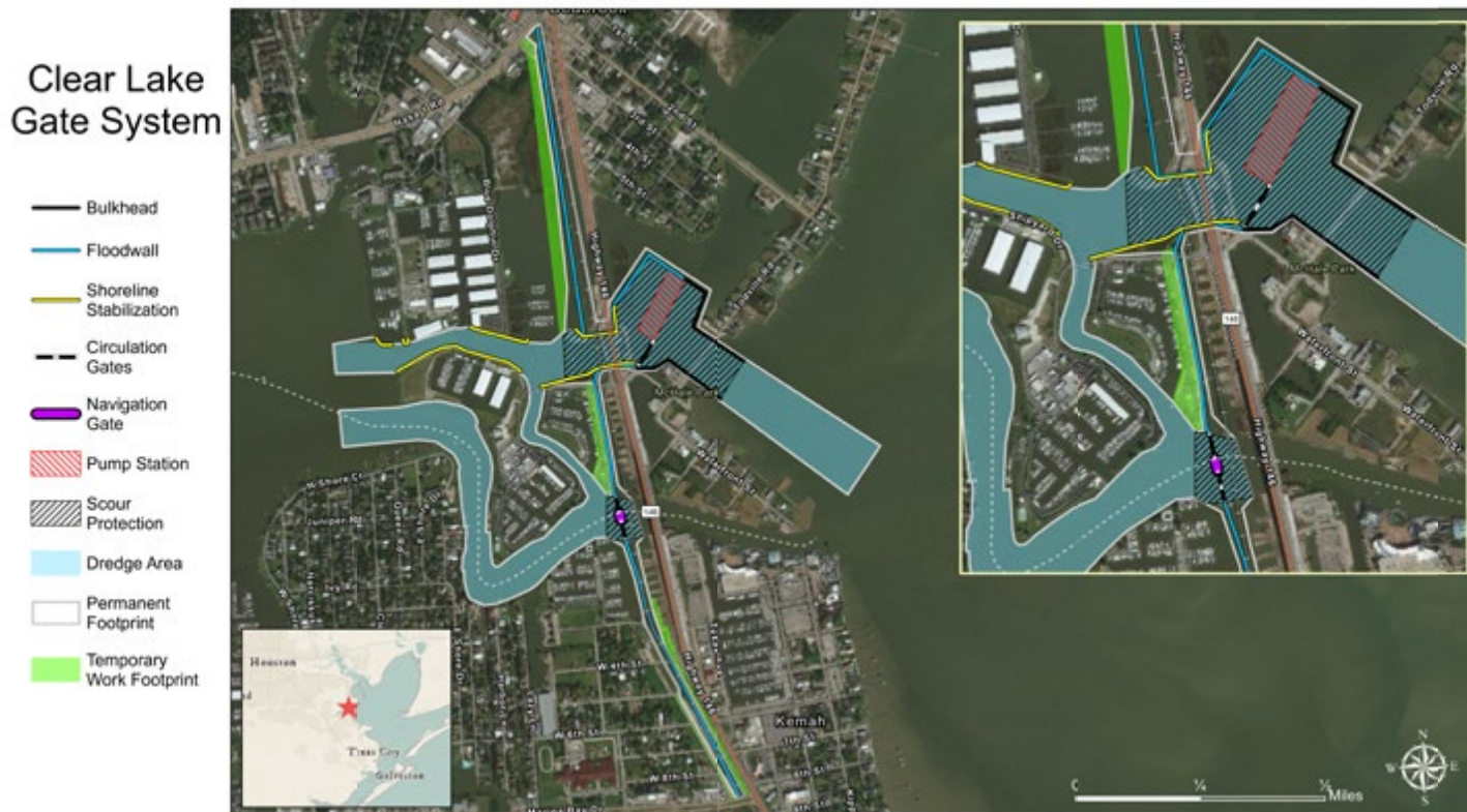
Figure 3.41: Clear Lake gate system and pump station
