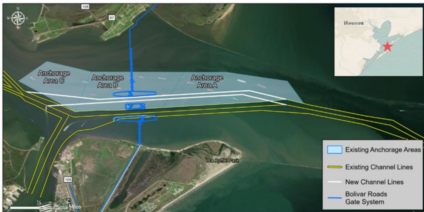
Figure 3.24: Bolivar Roads channel configuration
