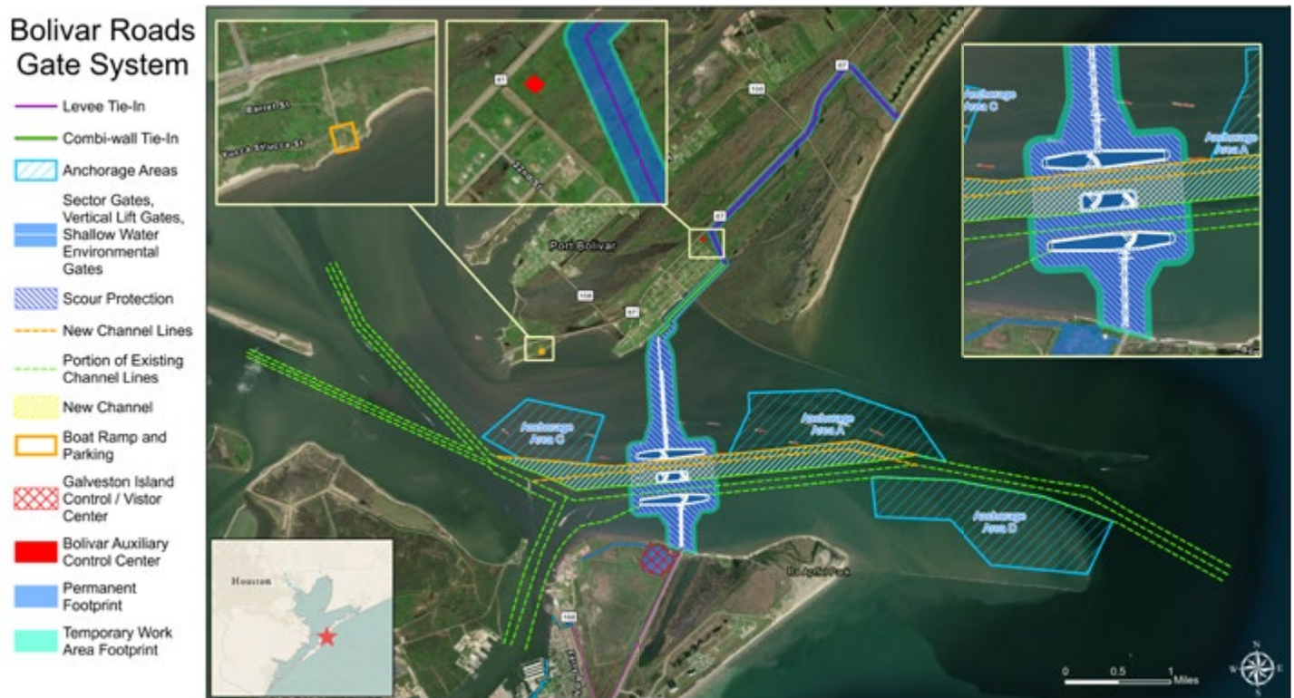
Figure 3.16: Bolivar Roads gate system - overview
