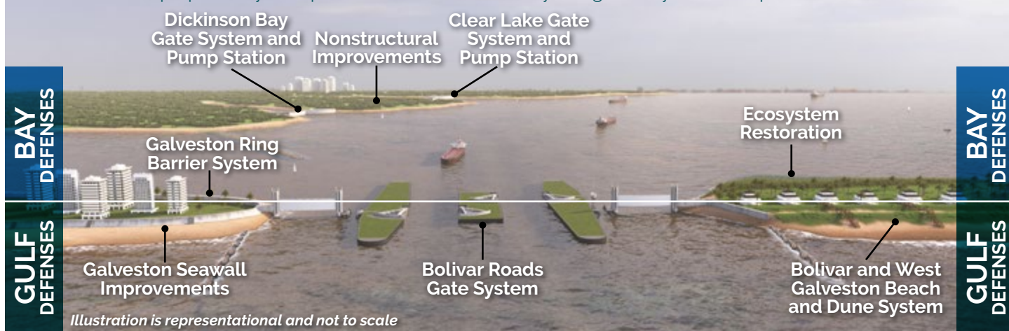
Figure 1.1: Examples of multiple lines of defense on the Texas coast
