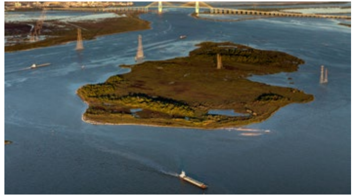
Dredge material from the Houston Ship Channel Expansion Channel Improvement Project may serve as source material for constructing select portions of the Galveston Bay Storm Surge Barrier
